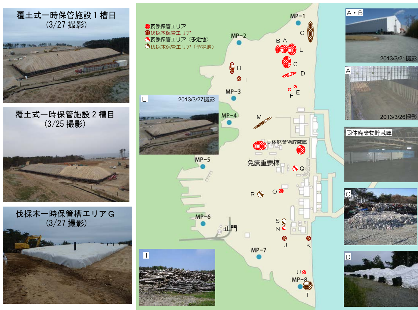
図8：ガレキ・伐採木の線量低減対策
