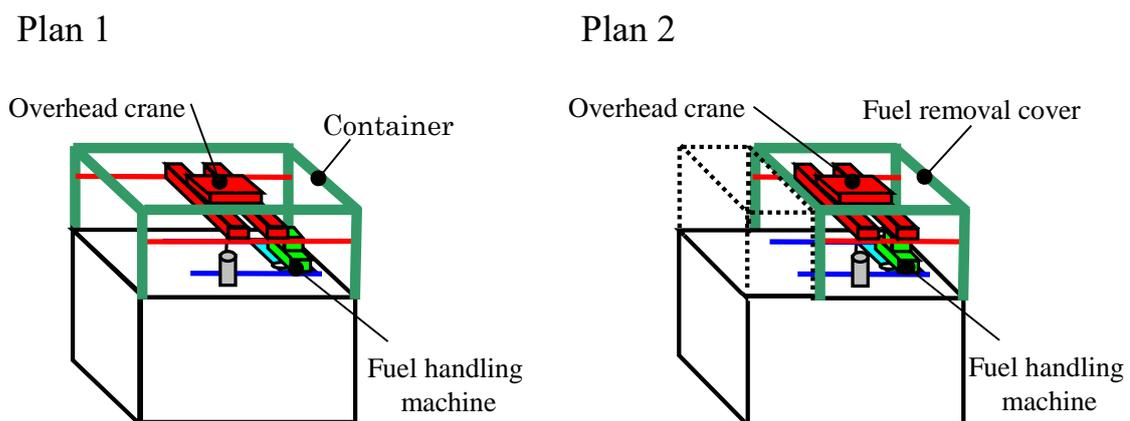
Figure 2: Fuel handling equipment of Unit 2 (conceptual illustration)
