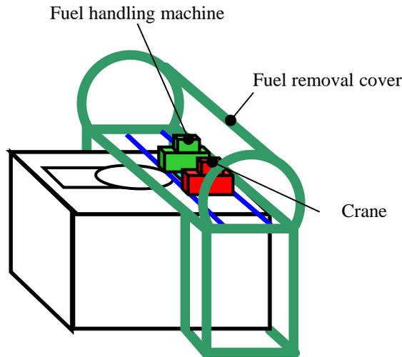
Figure 3: Fuel handling equipment of Unit 3 (conceptual illustration)
