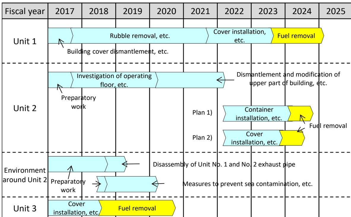
Figure 4: Plan of fuel removal from spent fuel pools of Units 1 to 3
