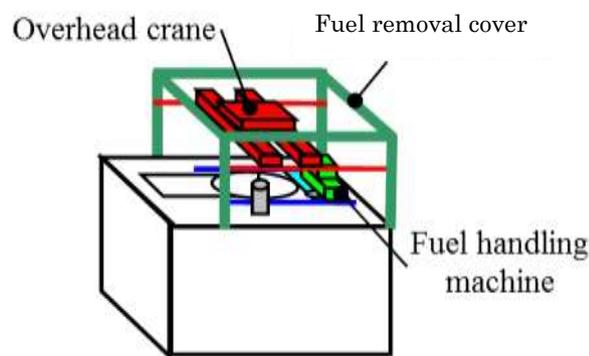
Figure 1: Fuel handling equipment of Unit 1 (conceptual illustration)
