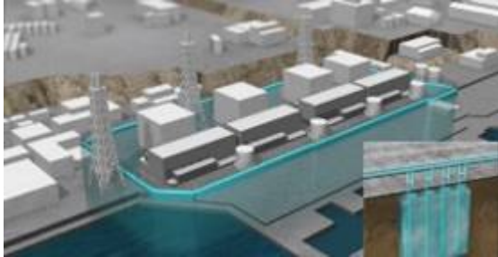
Figure 1: Land-side impermeable wall (Image)
