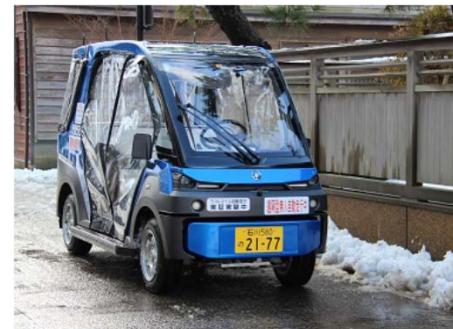
Demonstration of Automated Driving with no person in the vehicle
