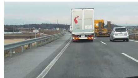
A low-speed vehicle blocks the lane together with platooning vehicles.
