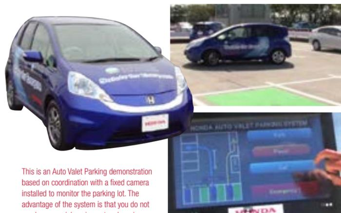
This is an Auto Valet Parking demonstration based on coordination with a fixed camera installed to monitor the parking lot. The advantage of the system is that you do not need any special equipment on board.
