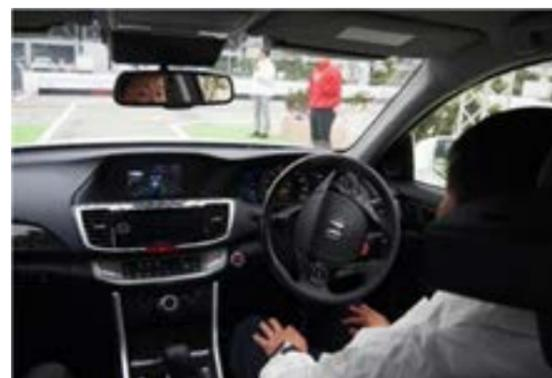
This is a driving demonstration simulating a public road. The system can respond even to the sudden appearance of pedestrians, with the use of a stereo camera, a millimeter-wave radar, and wireless communication with smartphones.
