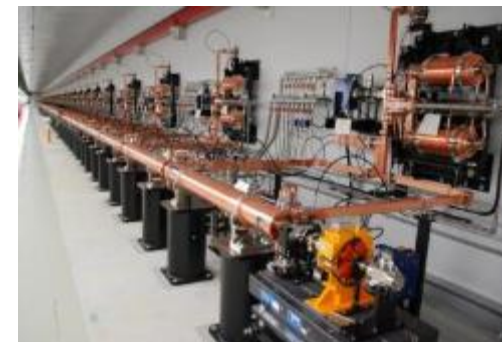
【Chart 3-7: C-band Accelerator which Accelerates Electrons to the Speed of Light】
