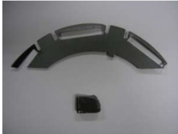
切断電磁鋼板+Nd磁石
