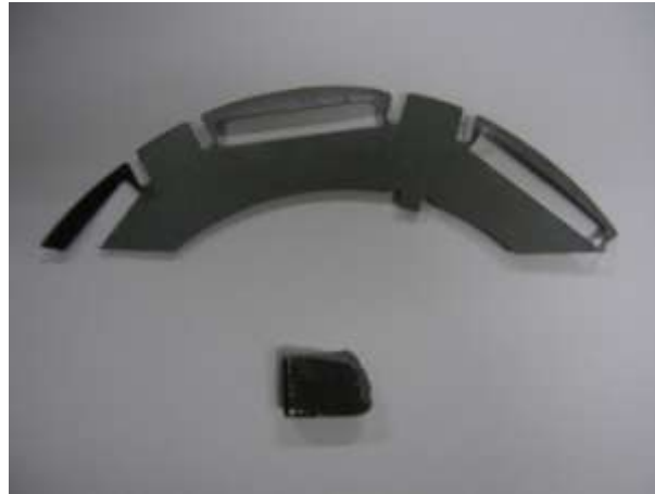
切断電磁鋼板+Nd磁石
