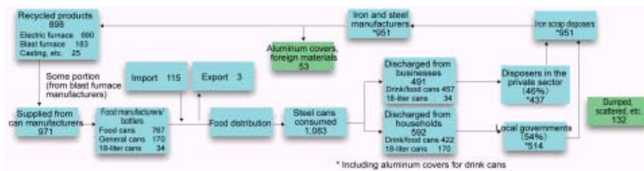
Fig. 49 Flow of Recycling of Steel Cans (estimate in 2001) (Unit: thousand tons)
