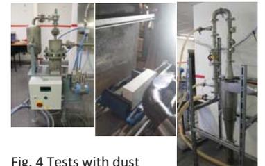
Fig. 4 Tests with dust collection devices prototypes
