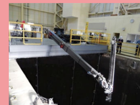
Robotic arm for trial retrieval
