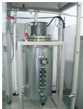
Leak detection experiment by using microphone array
