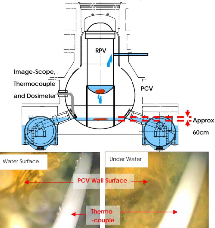
Fig.1: Internal PCV Inspection Results at Unit 2
