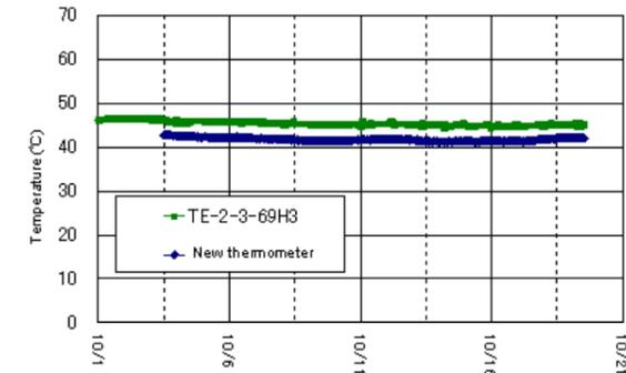
Change in the readings of the existing RPV monitoring thermometer (① TE-2-3-69H3) and the RPV alternative thermometer (② New thermometer)
