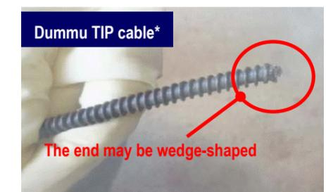
\* Cable used to check before installing the actual TIP detector during the plant construction
