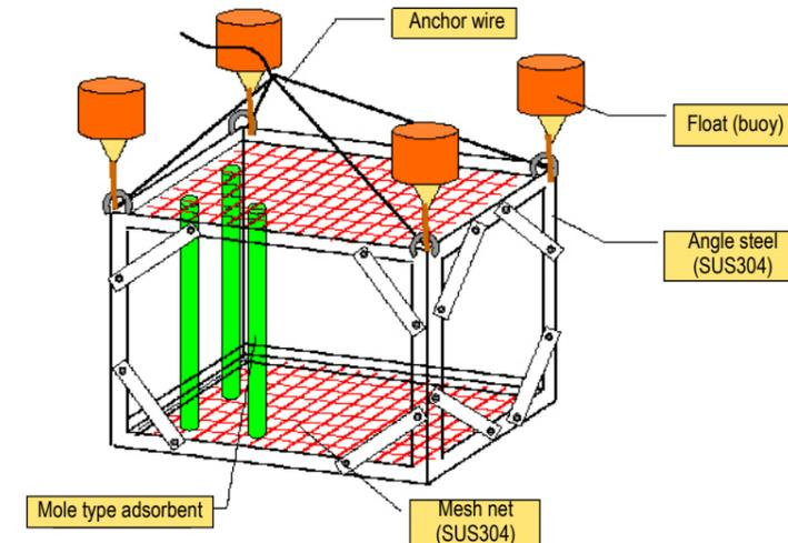
Figure 2: Fiber-adsorbent cleaning equipment
