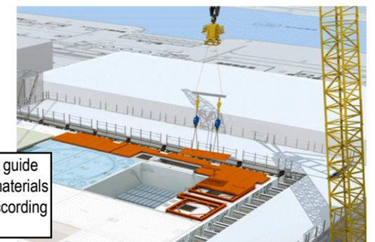
After installing the guide frame, shielding materials will be installed according to the frame
