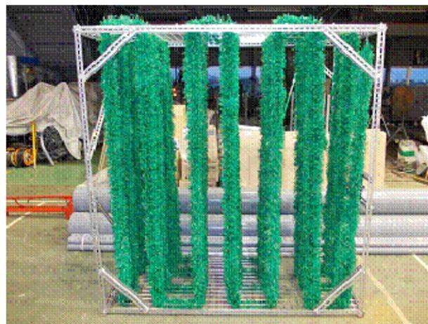
**Fiber adsorbent purification equipment**
