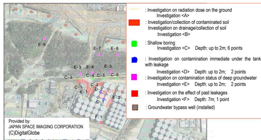
Figure 3: Investigation points around the tank
