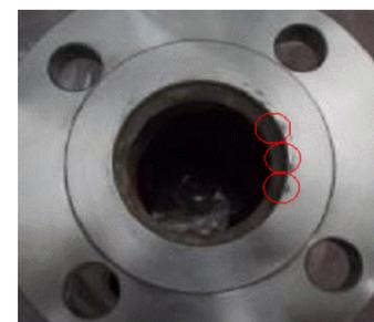
Tiny crevice corrosion identified at 3 spots
