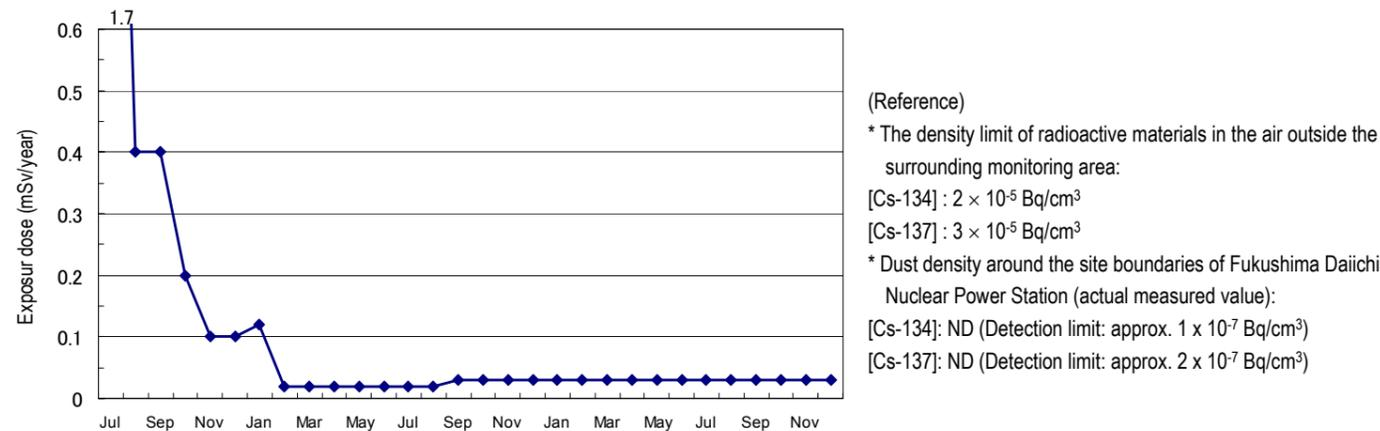
(Note) Different formulas and coefficients had been used to evaluate the radiation dose in the facility operation plan and monthly report. The evaluation methods were integrated in September 2012. As the fuel removal from the spent fuel pool (SFP) commenced for Unit 4, the radiation exposure dose from the Unit 4 has been added to the items subject to evaluation since November 2013.
