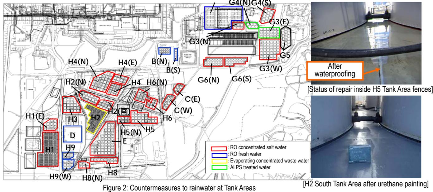
Figure 2: Countermeasures to rainwater at Tank Areas
