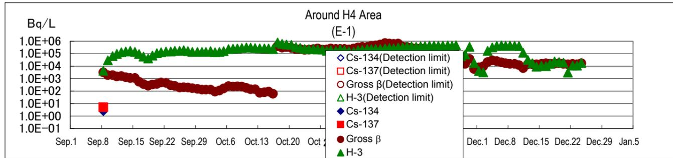
Figure 1: Radioactive material density of Observation Hole E-1
