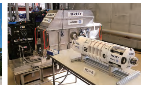
Marine robot for internal investigation of Unit 1
