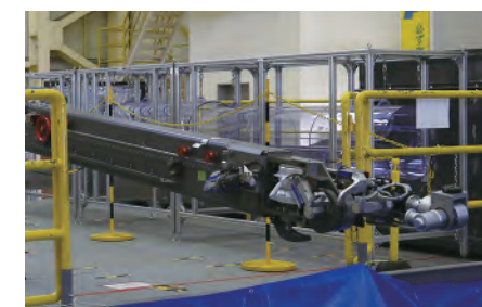
Robotic arm for trial retrieval
