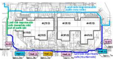
Closure parts of the land-side impermeable walls (on the mountain side)
