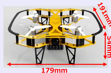
< Small drone used in the investigation in Unit 1 >
