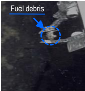
Gripping fuel debris with the end tool
