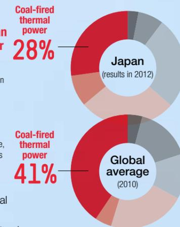
The ratio of thermal power generation to overall electricity generation in Japan rose to around 90% in FY2012. Of the electricity generated through thermal power generation, around 50% comes from LNG-fired thermal power generation. Worldwide, coal-fired power generation accounts for approximately 40% of overall electricity generation.
