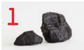
1 USC uses the fine coal combustion method. Coal transported to the plant is burned after being pulverized into fine powder with a grain diameter of around 70 microns.
