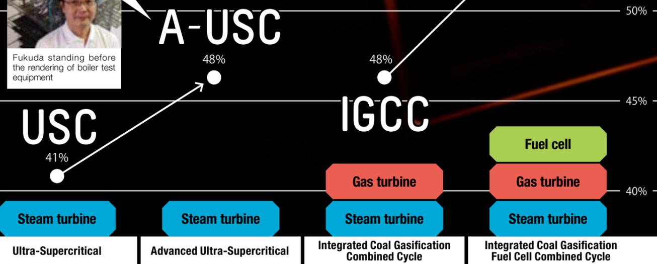
Generates steam within the boiler and uses the steam turbine to drive the generator. Increases the thermal efficiency by raising the steam temperature to around 600 degrees Celsius.
