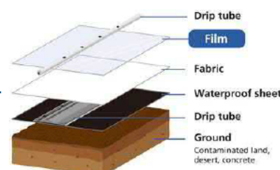
▲Simple and Affordable “Imec®” System consisting of fluid supply equipment and Cultivation Bed
