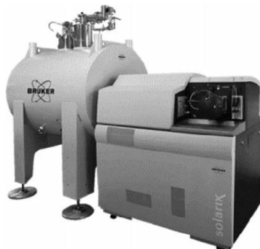
Fig. 3 Fourier Transform Ion Cyclotron Resonance Mass Spectrometry (FT-ICR MS)
