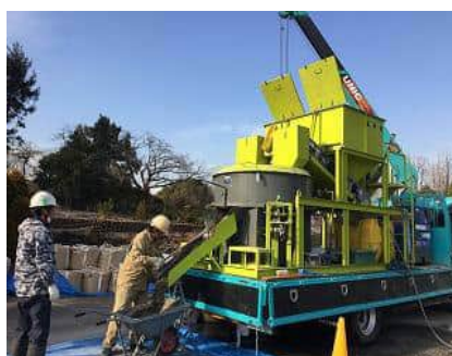
▲ Vehicle-mounted manufacturing plant (Mobacon)
