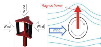
▲ Magnus x Vertical Axis Wind Turbine (left) and Magnus Effect (right)
