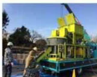
▲ Vehicle-mounted manufacturing plant (Mobacon)
