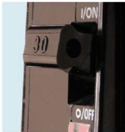
Ampere ratings molded into the handles of new (post 1999) breakers indicate the product is counterfeit.
