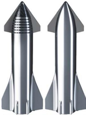
Figure 2: Starship crew (left) and uncrewed (right) configurations
