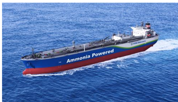
Figure 7 40,000m 3 type ammonia fuel ammonia carrier (Source: NYK)
