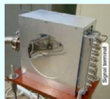
High precision absorbed dose to water measurement using graphite calorimeter
