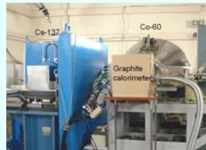
Co-60 gamma-ray absorbed dose to water was developed using a graphite calorimeter.
