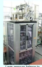
Large pressure balance to achieve high pressure standards
