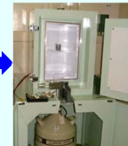
Gamma-ray spectrometry using germanium semi-conductor detector
