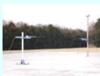
Dipole antennas in the standard measurement
