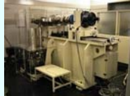
Developed 1 kN-m torque standard machine
