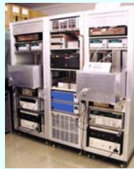
AC/DC difference measurement system
