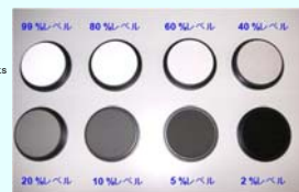
Example of standard diffuser plate traceable to national standard
