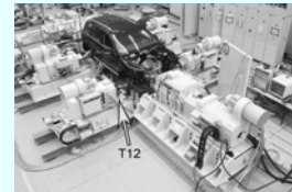
Power train measurement system for vehicles (Manufactured by HORIBA Europe GmbH) Source: S.Kuhn, Proc. XIX IMEKO World Congress, pp.351-355, Lisbon, Portugal, 2009.
