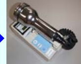
Calibrating a portable surface contamination meter using a large area source
