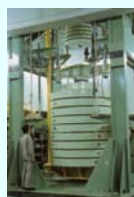
Mass adjustment and calibration for deadweights on a force standard machine (national measurement standard for force)
