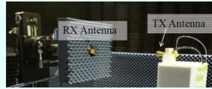
Millimeter wave antenna properties measurement using optical devices
