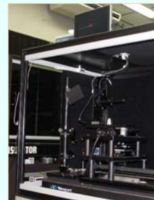
LED photometric calibration device developed by AIST
