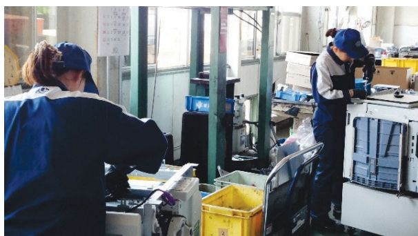
▲ Workers are dismantling OS equipment with a power tool
