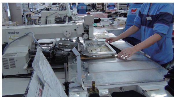
▲ Sewing operation using the large electronically-controlled automatic sewing machine
