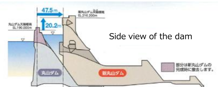
Strengthening flood control functions and increasing hydroelectric power generation by raising the dam height
