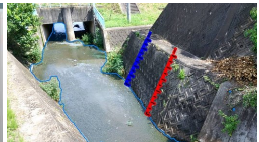
▲ The edge AI detects the water surface in the image and measures the water level.
