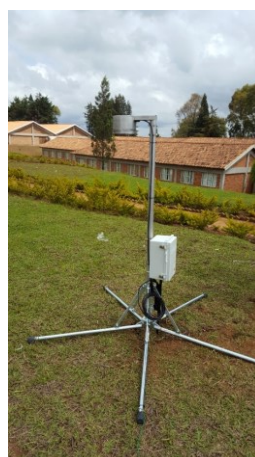
▲ (Sensor Signaling the Approach of Lightning)
