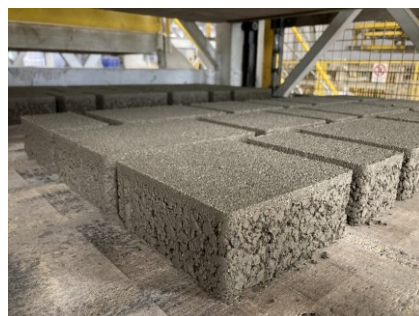
▲ Permeable blocks manufactured at block manufacturing plant
