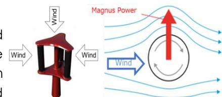
▲ Magnus x Vertical Axis Wind Turbine (left) and Magnus Effect (right)
