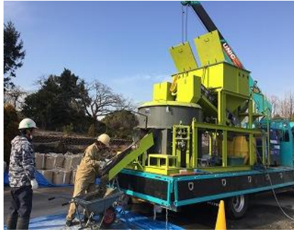
▲ Vehicle-mounted manufacturing plant (Mobacon)
