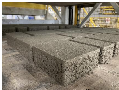
▲ Permeable blocks manufactured at block manufacturing plant
