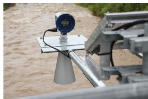
▲Example of Non-Contacting Radar Level Gauges Delivery to a River
