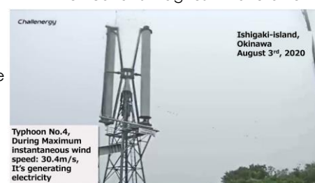
▲ Generated power at 30.4 m/s peak wind speed
