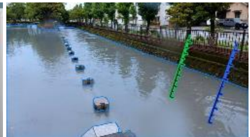
▲ The AI detects the surface of the water on the captured image.
