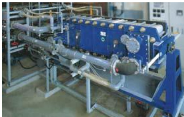
◀ Electro Dialysis Purification System
