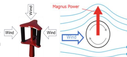
▲ Magnus x Vertical Axis Wind Turbine (left) and Magnus Effect (right)
