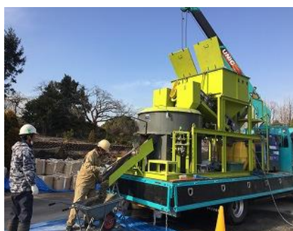
▲ Vehicle-mounted manufacturing plant (Mobacon)
