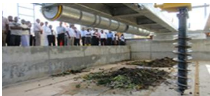
▲Screw-shaped Compost Plant “RA-X”
