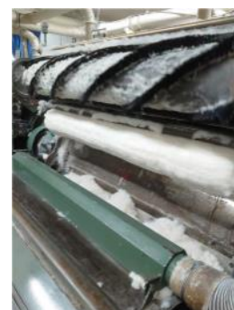
Reuse of flat strips (fallen cotton) at carding as blended cotton
