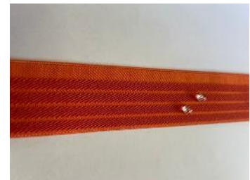
Highly functional waist elastic with water-repellent and water-absorbent yarns woven into uneven surfaces
