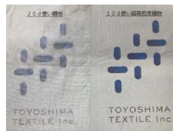
The transparently thin, ultra-high-density woven fabric
