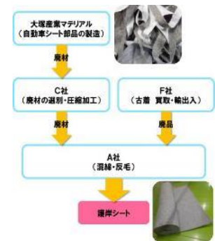
Manufacturing of revetment sheets using non-woven fabric materials
