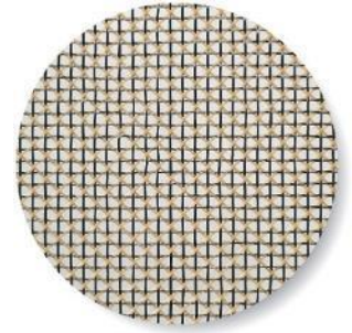
"Tetras", the world's only proprietary four-axis woven fabric
