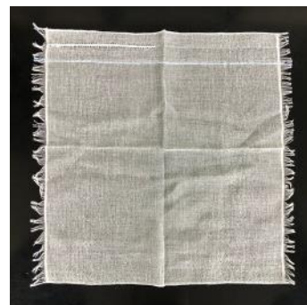
Threaded RFID tags and surgical gauze
