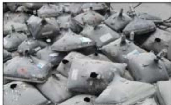
Broken CRTs awaiting land disposal after the copper yoke has been removed in Guiyu, China. © BAN
