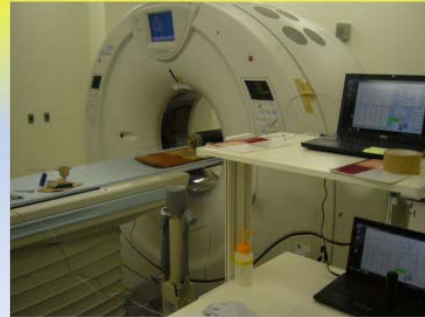
Visualization of MB CO 2 injection using X-CT
