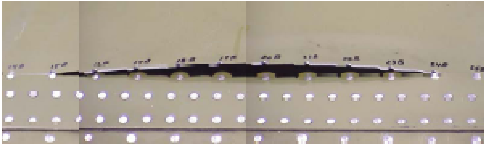
a. Crack in outer rivet row of lap splice joint
