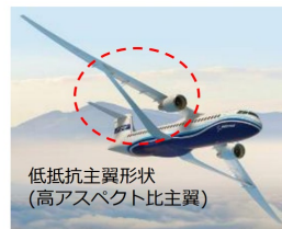
低抵抗主翼形状 (高アスペクト比主翼) 出典: Boeing https://www.boeing.com/features/2019/01/spread-g-our-wings-01-19.page
