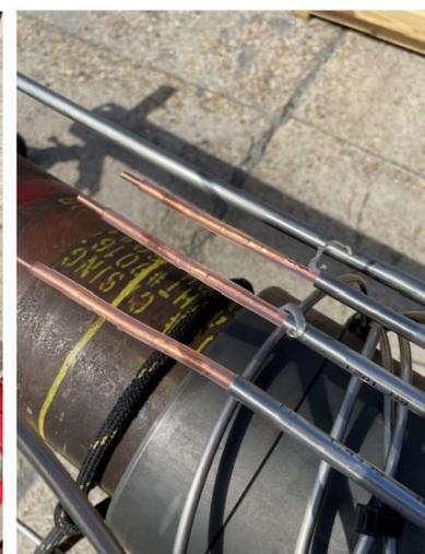
Figure 20. Damage to ESP leads after pulling adapter / hanger
