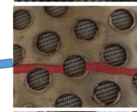
Mesh screen between base pipe and Shape memory polymer
