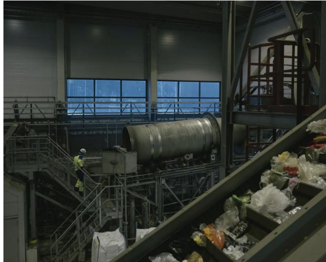
A scene at Fortum Waste Solutions Oy's circular economy facility in Häme, Finland on Dec. 14. In the facility, waste material collected from regular households is converted to clean plastic through Fortum's Eco Refinery—an automated sorting plant. Ingmar Björn Nolting for TIME
