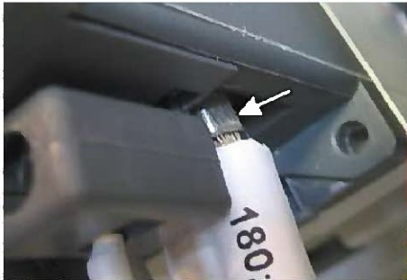
Figure 13-3: A maximum of 2 mm of the ferrule must be visible (in this photo more than 2 mm is visible!)
