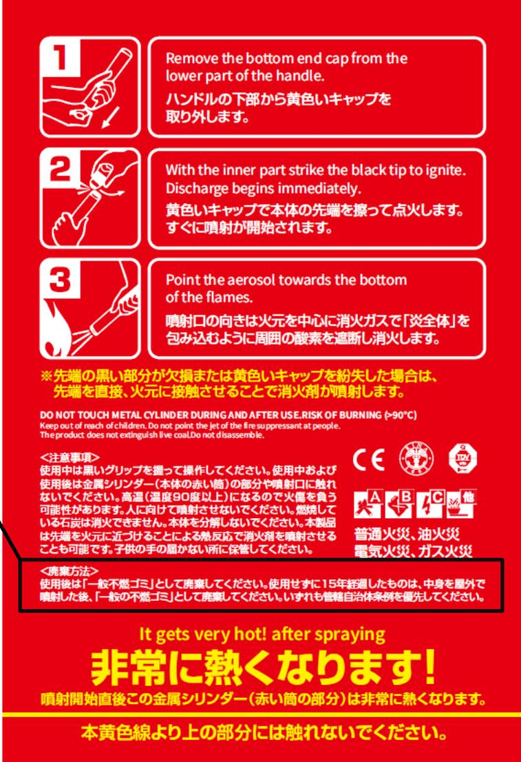
**1** Remove the bottom end cap from the lower part of the handle.
