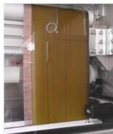
Lithiated anode electrode roll sheet especially for high energy density LiB etc
