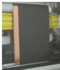
Anode electrode roll sheet
